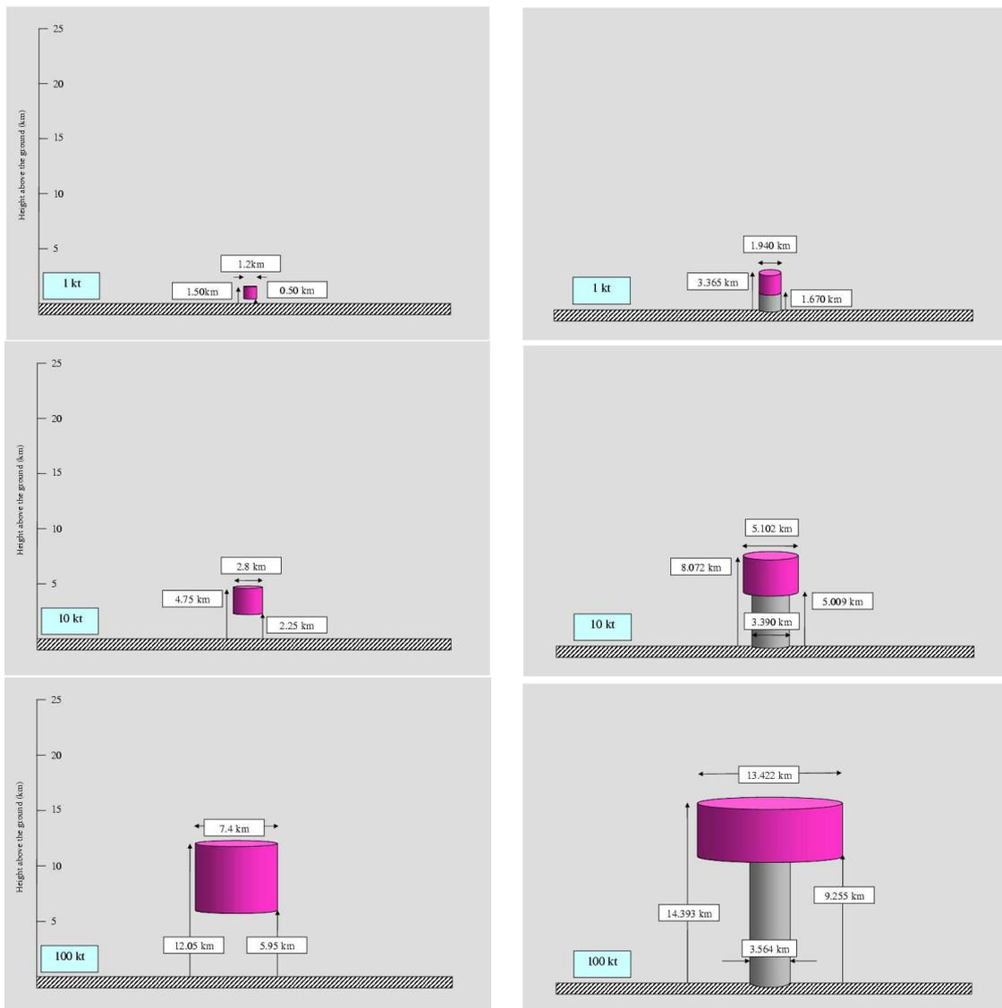
Figure 1. Initial shapes of the radioactive cloud shortly after explosion for 1, 10 and 100 kt yield. Cylindrical form to the left, mushroom to the right.
